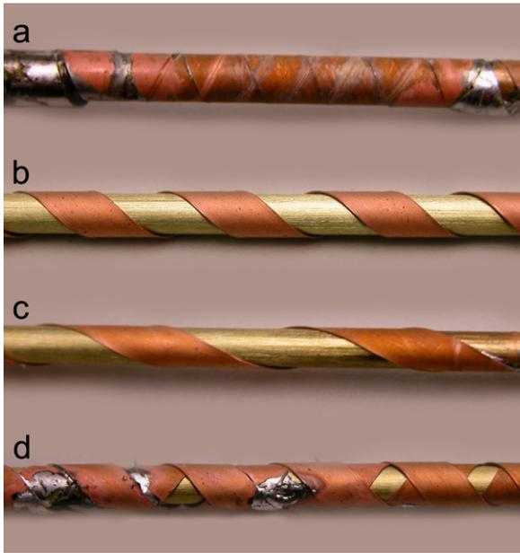
**Figure 2.** Prototype cables prepared by winding a single YBCO coated conductor around a brass former, 3.19 mm in diameter, with twist pitch (a) 9 mm, (b) 20 mm, (c) 40 mm, and (d) by winding two layers of conductors with 18 mm twist pitch.
