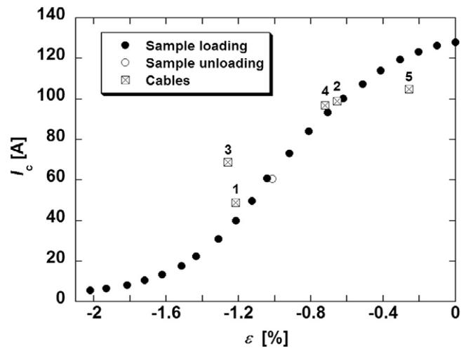
**Figure 1.** Critical current as a function of axial compressive strain at  $76\ \text{K}$  of a YBCO coated conductor that is soldered on a brass bending beam. The applied strain is measured directly on the surface of the sample with a strain gage. The critical currents at the calculated strain state of prototype cables (numbered) are included (below, table 1).
