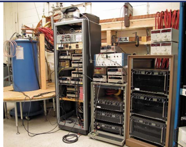
Figure 3: Facility to test CORC cables at currents in excess of 10,000 A in a background magnetic field
