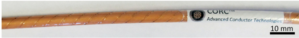
Figure 3. The CORC ® cable containing tapes with 38 \mu\text{m} thick substrates. The 6 mm diameter cable contains 50 tapes wound in 23 layers.
