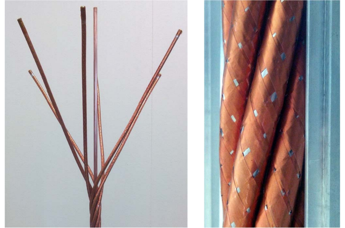
Fig. 3. (Left) Photograph of the winding process where the six dummy strands are wrapped with a central copper tube. (Right) Photograph of the twisted strands positioned inside the conduit.
