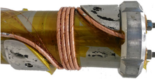
Fig. 1. CORC wire wound into a 5 turn solenoid on the stainless steel sample holder prior to applying mechanical reinforcement.
