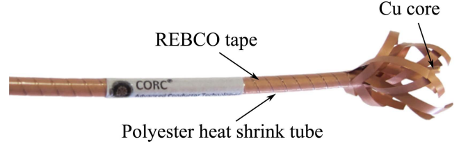
Figure 1. The commercial CORC ® wire manufactured by Advanced Conductor Technologies, LLC. A polyester heat shrink tube encapsulates multiple layers of REBCO tapes helically wound on a Cu core.
