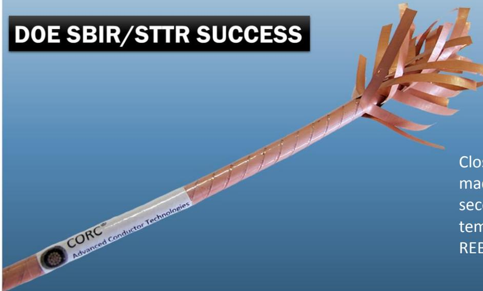
Close-up of the CORC<sup>®</sup> cable made from individual tapes of second generation high-temperature superconductor REBCO.
