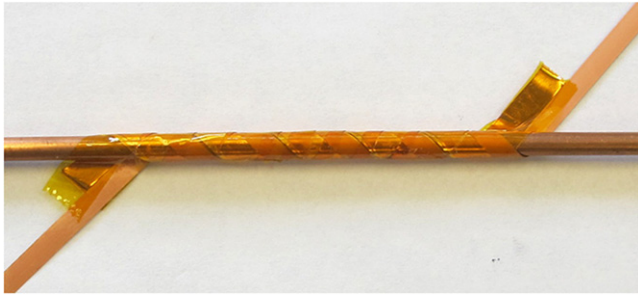
Figure 1. A 3 mm wide superconducting tape wound onto a 2.8 mm diameter former. A 3 mm wide copper tape is wound in parallel to the superconducting tape to ensure a constant winding angle close to 45°.
