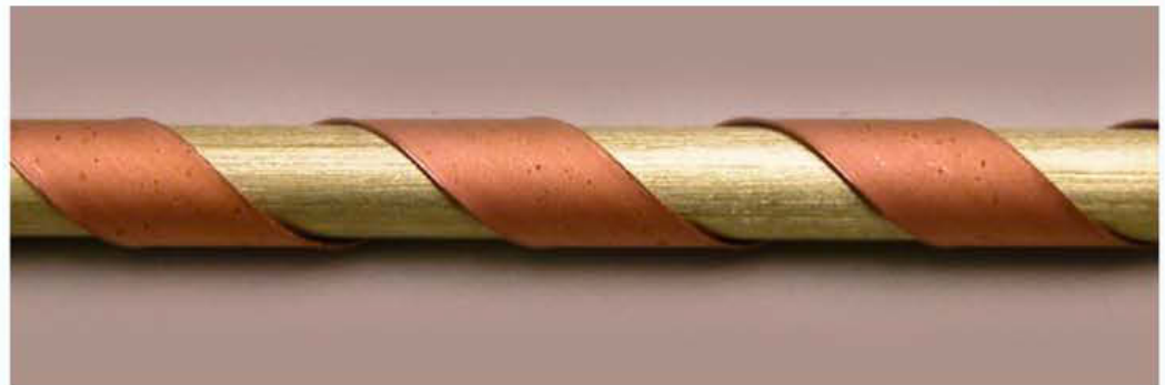
Single tape wound into a CORC® cable
