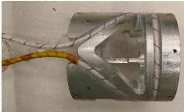
CORC ® cable tested at 100 mm diameter (2011 – 2015)
