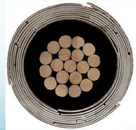
Single tape wound into a CORC® cable
