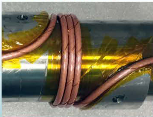
CORC ® wire tested at 60 mm diameter (2016 – )
