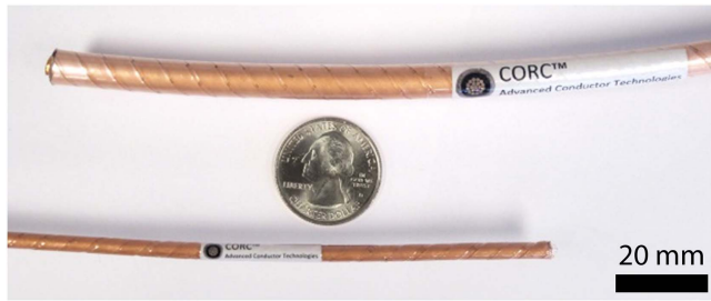
Figure 1. 7 mm diameter CORC® cable (above) made out of 4 mm wide REBCO tapes with 50 \mu\text{m} thick substrates compared to a 3.6 mm diameter CORC® wire (below) made up of 2 mm wide tapes with 30 \mu\text{m} thick substrates.
