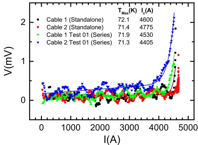
**Figure 14.** *V*-*I*-curves of the two poles of cable CORC<sup>®</sup>-3 at a maximum temperature of about 72 K measured on the connector at the outlet side of the cryostat. The poles were energized separately when standalone and together when connected in series. Lines are fits used to determine  $I_c$  using equation (1).
