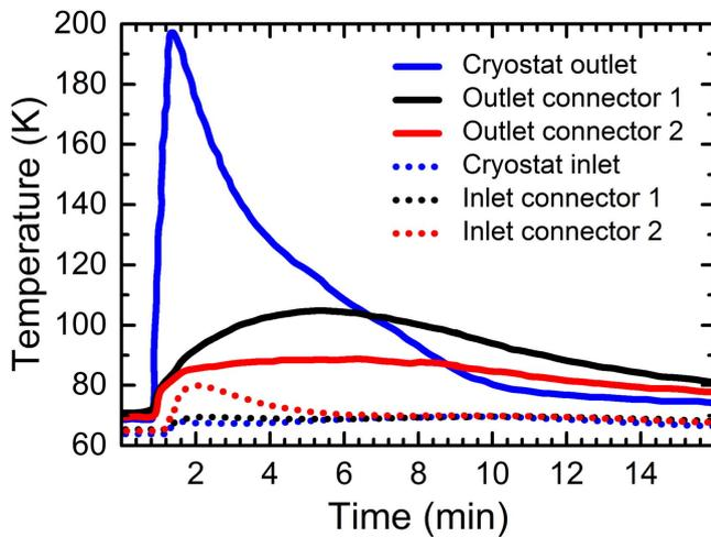
**Figure 17.** Temperature as a function of time of the two-pole operation of cable CORC<sup>®</sup>-3 during the overcurrent event that lasted 2 s.
