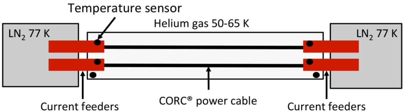
Figure 6. A schematic of the test configuration of the two-pole CORC® cables in helium gas.
