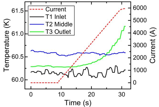
**Figure 13.** Temperature as a function of time at different operating currents of cable CORC<sup>®</sup>-2 in the short helium gas cryostat. The current was increased at a constant rate of about  $300 \text{ A s}^{-1}$ .
