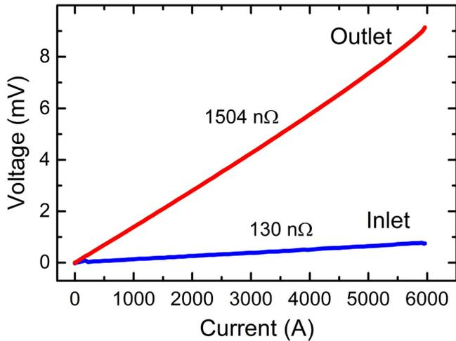
**Figure 11.** *VI*-characteristic of the copper connectors between the CORC<sup>®</sup> cable terminals and the feeders cables when operated in helium gas at 60 K for both connectors.
