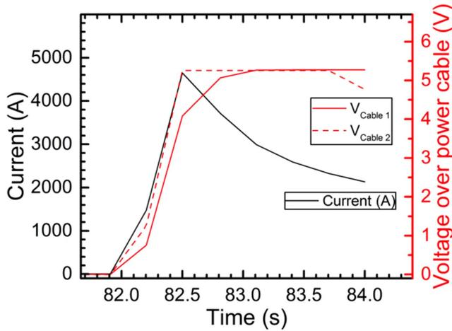
**Figure 16.** Current and voltage as a function of time of each of the two poles of cable CORC<sup>®</sup>-3 during the overcurrent event.
