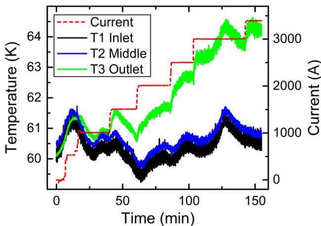
**Figure 12.** Temperature as a function of time at different operating currents of cable CORC<sup>®</sup>-2 in the short helium gas cryostat. The current was increased stepwise, while it was held constant for about 15–20 min between steps.
