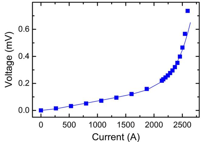
**Figure 10.**  $VI$ -characteristic of cable CORC<sup>®</sup>-2 measured at 76 K. The solid line is a fit to the data according to equation (1).
