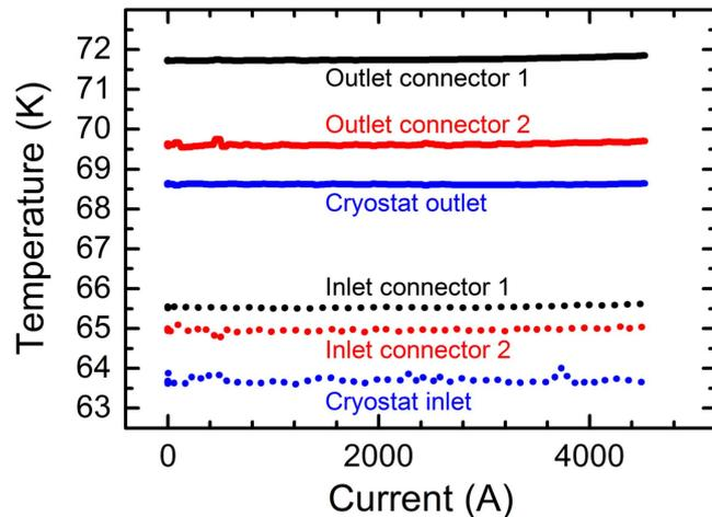
**Figure 15.** Temperature as a function of current during the two-pole operation of cable CORC<sup>®</sup>-3.
