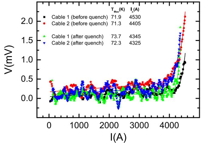
**Figure 18.**  $V$ - $I$  curves of the two poles of cable CORC<sup>®</sup>-3 when connected in series before and after the overcurrent event.
