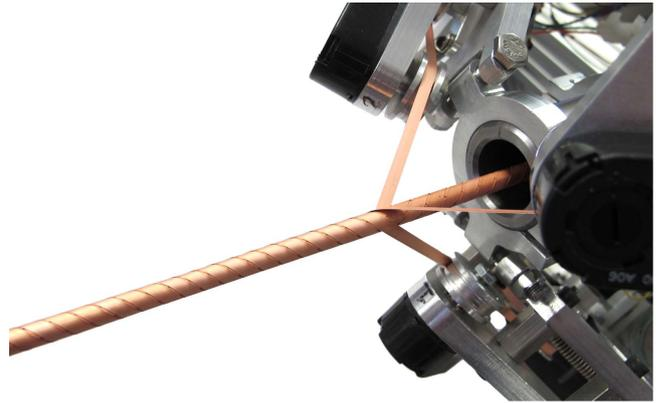
**Figure 1.** Winding head of the custom CORC<sup>®</sup> cable machine containing three tape spool holders.
