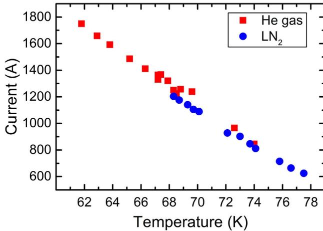
**Figure 9.** Temperature dependence of  $I_c$  of cable CORC<sup>®</sup>-1 measured in both sub-cooled liquid nitrogen and pressurized helium gas.
