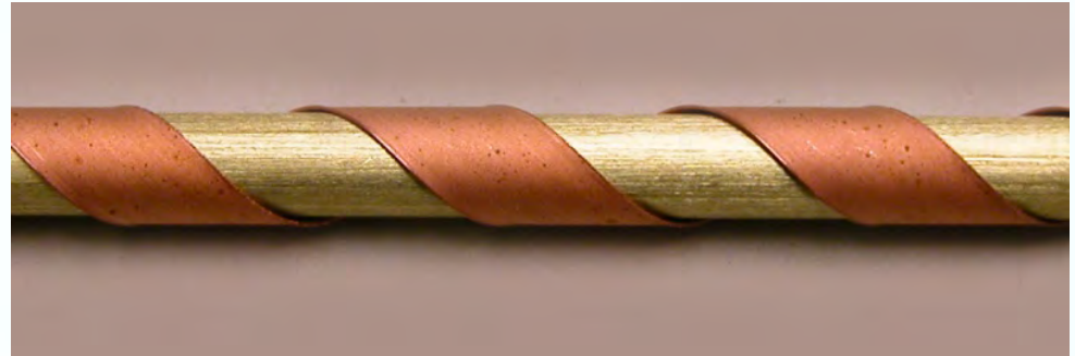
Single tape wound into a CORC® cable
