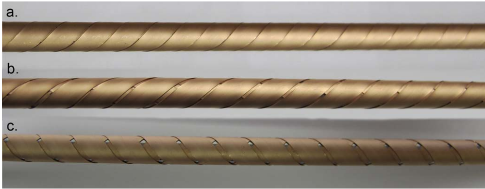
Figure 1. (a) Sample CORC®-1 wound without gaps between the tapes, (b) sample CORC®-2 containing 0.5 mm wide gaps, and (c) sample CORC®-4 containing 1 mm wide gaps.
