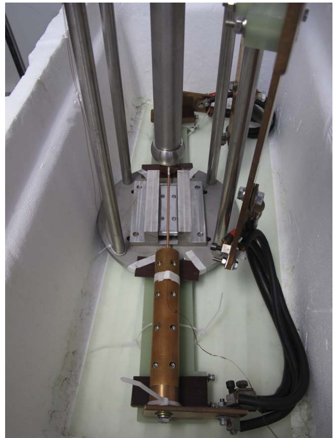
Figure 4. A CORC® wire being installed into the load frame, before the top anvil is placed on top of the sample.
